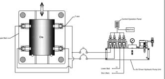
T-slot mounted single acting rocker clamps ERC, hollow rams ECA or MHC or T-slot clamps MTC with split safety circuit on the upper bed and one circuit on the lower press bed and one circuit for the single acting die lifters.
