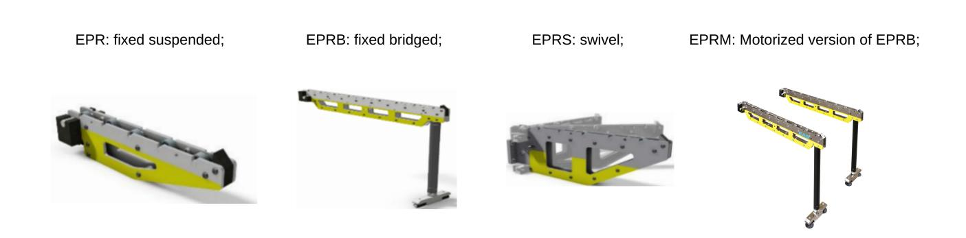
The EAS pre-rollers extend the side opening of a machine to enable a quick and safe horizontal manual mold or die transfer. Always mounted as a set, EAS pre-rollers are equipped with needle roller bearings with hardened steel surfaces to offer a high load capacity. The die or mold is loaded onto the pre-rollers with the help of a cart, forklift or crane.
