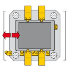
Horizontal load mold change with non powered rollers
