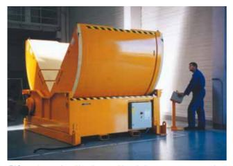
EAS can also supply mold turning or mold manipulators to turn your expensive molds 90 degrees for transport or storage in a different way.
