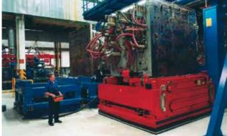
For extreme heavy molds as at this container manufacturer EAS installed this air floating system in combination with storage systems, a 3400 t and a 6000 t injection molding machine as well as an EAS inspection unit. The car can handle up to 150 t molds and the change over time is less then 30 minutes
