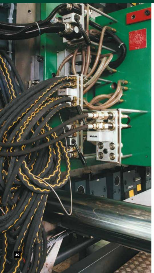
Simple and quick leak-proof connections of several water, air, oil and electrical circuits. EAS can provide you with a complete range of mono couplers as well.
