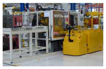
Electric driven  $2 \times 2$  ton mold change car serving several machines and storage systems.
