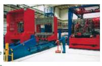
mold. Hydraulic core pulling cylinders are actuated in sequence with the opening stroke. Easy and safe maintenance without a huge overhead crane enables this customer to deal with transport and maintenance of very large molds.
