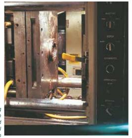
A clamping adapter plate is mounted to each SPI platen
