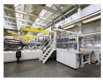
A table for 1 x 15 t mold with on one side the rollers with mold guidings, while on the other rollers molds with different dimensions can be placed. This table has a fixed operation panel. This table also features two guides to enable the crane operator to position the mold easily.
