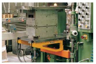
Mechanical clamps mounted on a special plate with spring loaded mold lifters and an isolating plate as well as a set of pre-rollers make this mold change on this Duroplast press a simple job.
