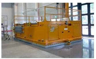
Air floating solutions can be very attractive for smaller mold handling requirements. It can also be combined with an electric drive system to travel longer distance. The operator can walk behind or even sit on board. Contact EAS for very creative solutions to your mold handling problems.
