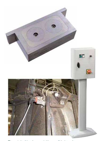
The control unit is only connected in case of closing and opening of the mold. A new electric pulse will de-magnetize the system, releasing the mold cover and clearing the clamping surface of any magnetic flux. After a magnetizing sequence, each square pole becomes either a North or a South Pole - and is again neutralized after having been de-magnetized.
