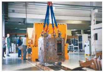
This turning unit is for molds up to 20 t and is remote controlled. EAS can supply these units up to 100 t mold weight.
