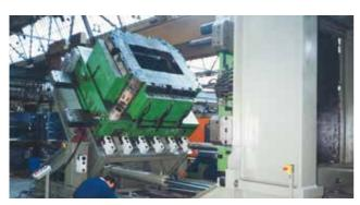
For a well known German manufacturer of plastic containers EAS equipped several large injection molding machines up to 6000 t with an adaptive hydraulic clamping systems, an air cushion mold change car, several mold storage racks and an inspection unit for molds up to 100 t.
