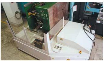
$1 \times 20 t$  with a combination of electric drive and air cushion floating for exact positioning in front of the machine, storage and inspection unit.
