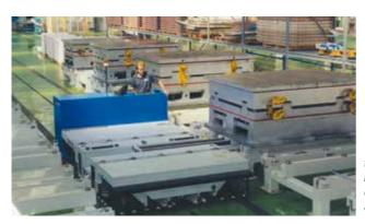
This electric driven mold change car for a large vertical press can bring the molds far away from the press to a special mold storage area. The molds can be stored left and right of the electric driven car. The driver has a camera and a monitor for exact positioning the car into the press. Changing and store molds between 10 and 20 t is in this way simple, fast and safe.
