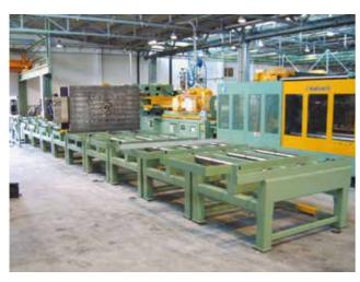
Mold storage racks in combination with a mold change car on rails. One of the storage racks is equipped with multi couplers and is serving as a pre heating station.
