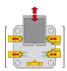
Vertical load moud change solution with, movable clamps. Clamps are moved manually or with hydraulic cylinders.
