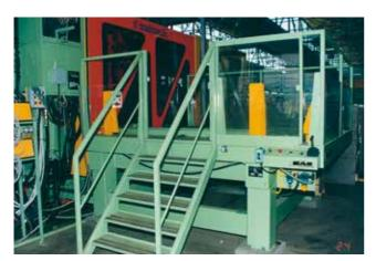
On an Italtech 1000 t injection molding machine EAS delivered the horizontal hydraulic adaptive clamping systems and a mold change table for molds of maximum weight of 40 t. Guides on the table allow the crane driver to easily position the large mold in a simple way on the table. An air driven push-pull spindle device moves the mold in and out the machine. All water, hydraulic and electric connections are made with manual multi coupler systems.
