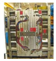
Two standard manual multi couplers with 12 water connections, a special manual multi coupler with 5 electric connectors for signals and heating purposes and one special manual multi coupler for hydraulic core pulling connections are mounted on these 40 t molds. The fluid and electrical connections are done within 3 minutes and without leakage of water or oil, which keeps the area very clean.
