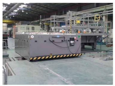
EASchangesystems tables and cars are build op from a modular design. Moldweight range from 5 t till 100 t. EAS installation at the customer.
