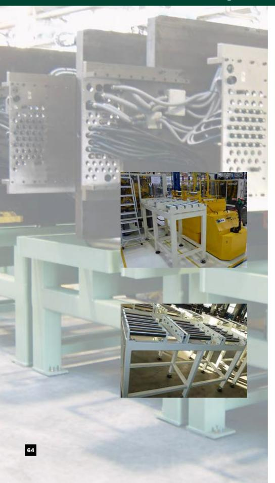
EASchangesystems offers a wide range of mold and die storage systems. These are simple roller beds for horizontal mold storage. They can be manually operated of fully automated.
