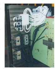
A manual multi coupler with several electrical connectors for heating and sensor signals.
