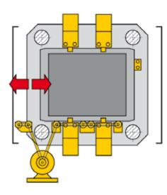
Horizontal load mold change with powered roller transfer
