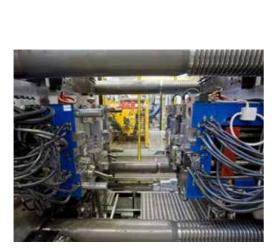
When molds are to be changed horizontally, clamps are positioned horizontally between the tie bars. The platens are equipped with rollers that allow the mold to roll into the press from a mold changing cart or table.
