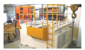
Space is very limited around the machines at this automotive supplier, two air floating cars for 1 x 20 t molds are used to change molds in less then 15 minutes.
