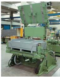
MOD wedge clamps were integrated in a specially designed ring for this special "Ringwalz" machine to produce automotive wheel frames. Due to the self-locking feature of this clamp, hydraulic pressure is not required after clamping or during the rotational movement of the ring.
