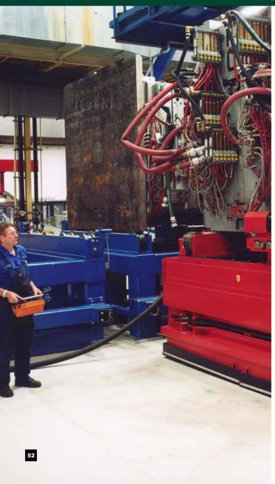
Air floating cars actually float on air film like a hovercraft and are therefor very flexible in moving around pillars or in restricted areas and can carry very heavy loads.
