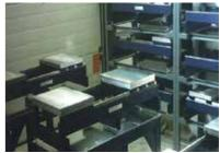
The standard units are all 1200 mm long, 580 mm wide and 275 mm high. The two turning platforms are  $350 \times 500$  mm. Optionally the units can be placed on a higher table for easier access or if you have other requirements such as clamping solutions.
