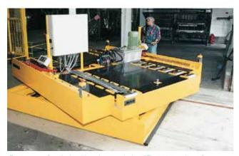
For a range of vertical mold carriers, producing different internal part for a well-known car manufacturer in Germany, the space in front of the mold carrier was very limited. A special designed electric driven car on rails was developed to overcome these difficulties.
