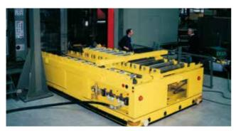
A 110 t mold is transported from its storage system to the injection molding machine or inspection unit. This customer, a producer of large plastic container, had no overhead crane available for such heavy weights and this solution enables them to change these molds within 35 minutes. The push pull mechanism is a simple spindle device, which pushes or pulls the molds in or out the large twin machine
