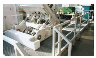
A German supplier of washing machines uses this inspection unit with two tilting platerns for 20 t molds. The loading and unloading of the molds is done by an electric driven and air floating mold change car. The unit can also simulate core pulling movements and ejector couplers movements.
