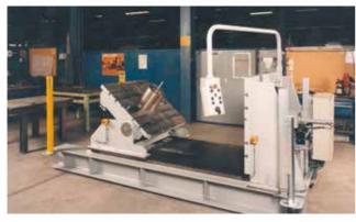
A small unit for molds of 2 t and with tilting platen. The control panel can be move around the unit by the operator. Safety mirrors as well as safety mat are also installed on this unit.
