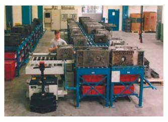
These horizontal mold storage systems are loaded and unloaded by means of electric driven mold change cars, on which either manual or automatically molds are placed. Underneath the molds is room for other mold related equipment.
