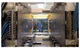
This 2700 t injection molding machines with horizontal loading, has standardized multi couplers on the movable and fixed side of the machines. Connections for cooling water, hydraulics for core pull cylinders and electric for heating and signals, are automatically connected and disconnected. This connection takes less then 30 seconds. All couplers feature the leak proof couplers, keeping floor and envirement clean.
