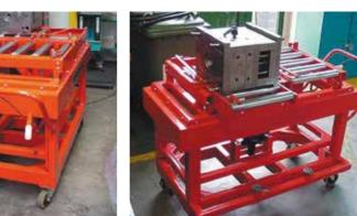
The molds are pushed and pulled manually.
