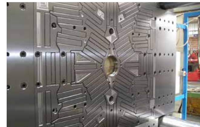
Pressmag HP on a 32000 kN (3200 t) machine
