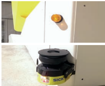
Laser scanner and warning lights
