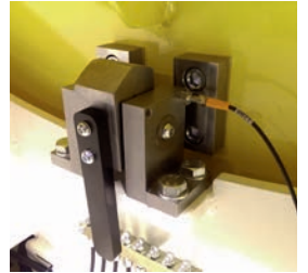
3 locking positions (0 ° -45 ° -90 °) with monitoring
