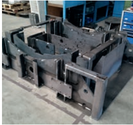
Laser cut modules
