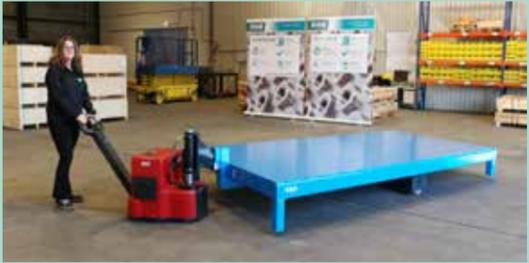
The truck is maneuvered into position and the hydraulic cylinder lifts the hook into the cradle on the trailer. The hydraulics are powerful enough to lift the trailer. Both parts are mated, making the truck and trailer as one. The additional load on the drive wheel of the truck ensures enough friction to move the load. When the final position is reached, the hook is lowered and the truck can be removed, ready for use on another trailer. No waiting time and optimum use of your truck.
