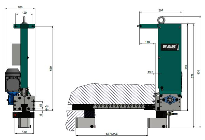
\*Note: dimensions may vary on the type of clamping cylinder.
