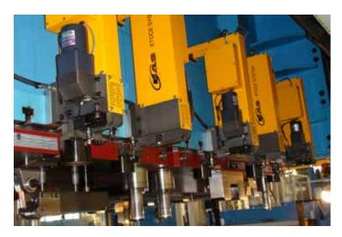
Travelling die clamps are commonly used on large stamping presses with various die sizes. These clamps allow automatic clamping of different sizes of large dies, especially on the slide. The slide is usually mounted with eight to sixteen of these clamps.
