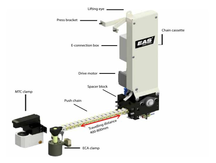
The EAS Electric driven Travelling Die Clamp (ETDCE) is a motor driven unit to move a hydraulic clamp through the T-slot of the upper bed of a press.
