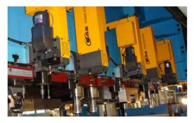
Travelling Die clamps are commonly used on large stamping presses with various die sizes. These clamps allow automatic clamping of different sizes of large dies, especially on the slide. The slide is usually mounted with eight to sixteen of these clamps.
