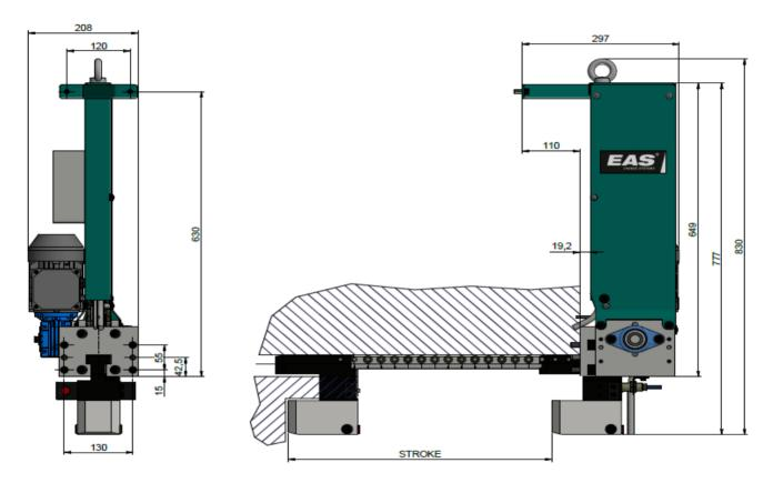
\*Note : dimensions may vary on the type of clamping cylinder.
