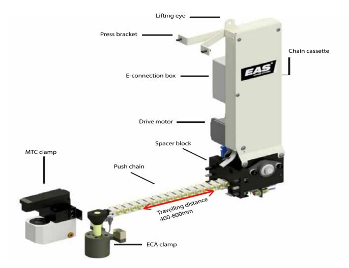
The EAS Electric driven Travelling Die Clamp (ETDCE) is a motor driven unit to move a hydraulic clamp through the T-slot of the upper bed of a press.
