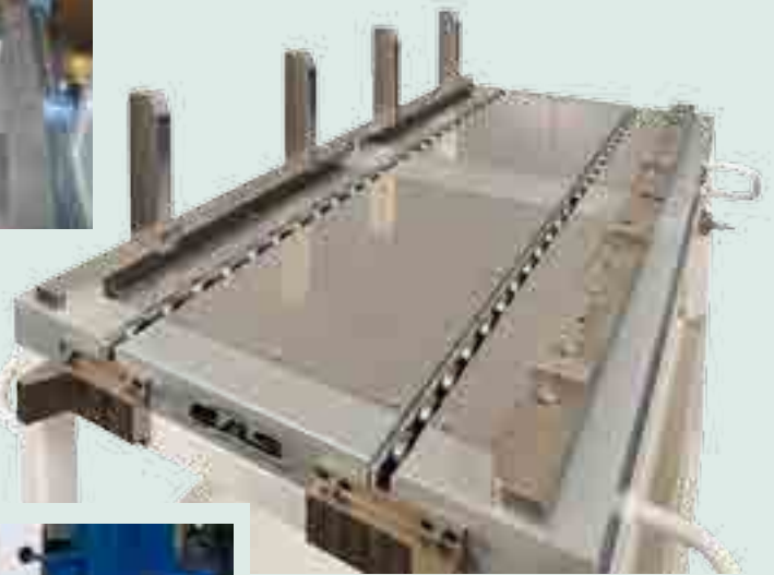
Die change car equipped with air operated die lifters with rollers and side guidings.
