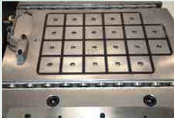
Bolster plate with side guiding die stop and air die lifters. Pressmag SP100 system with resin sealing.
