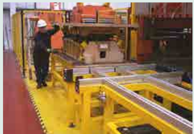
After tool is positioned with the help of die lifters the die lifters are removed and replaced in the same T-slot by MTC clamping cylinders.
