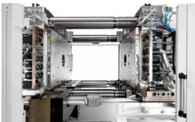
Pressmag LP on a 9000 kN (900 t) machine
