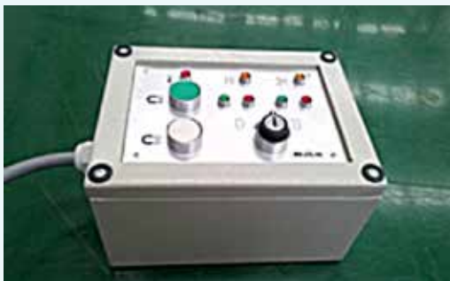
IL1 Control Unit
