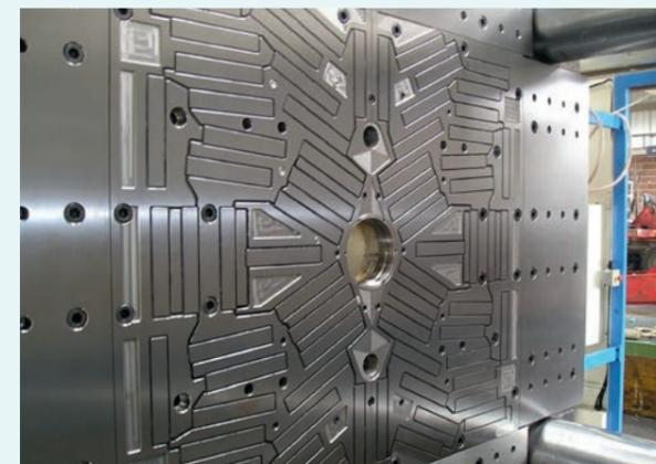
Pressmag HP on a 32000 kN (3200 t) machine
