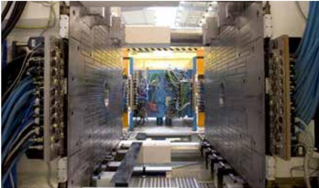
*This 2700 t injection molding machines with horizontal loading, has standardized multi couplers on the movable and fixed side of the machines. Connections for cooling water, hydraulics for core pull cylinders and electric for heating and signals, are automatically connected and disconnected. This connection takes less then 30 seconds. All couplers feature the leak proof couplers, keeping floor and envirement clean.*
