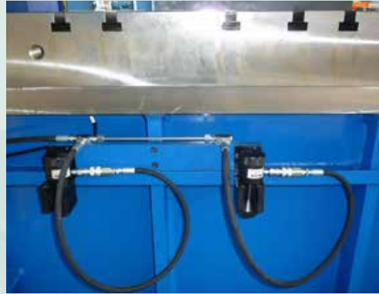
Pull cylinders on bolster with parking stations
