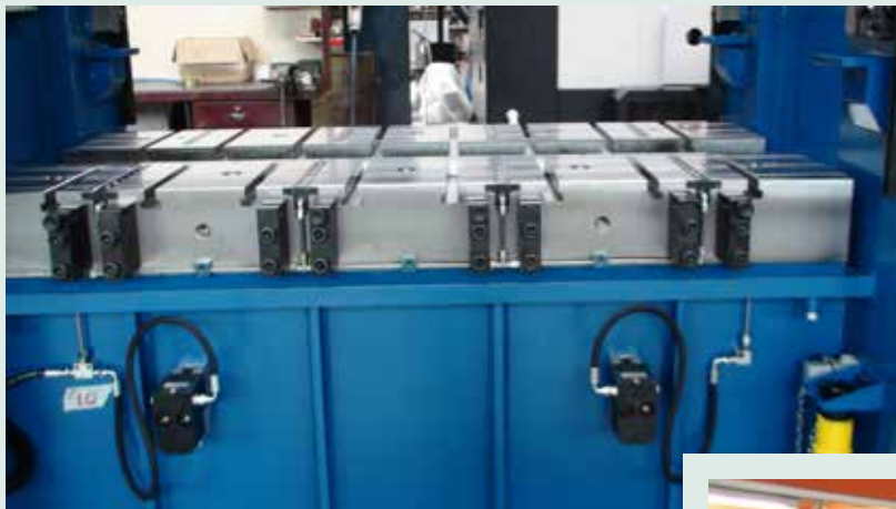
Bolster with air operated die lifters, pre rollers, ECA cylinders and parking stations.
