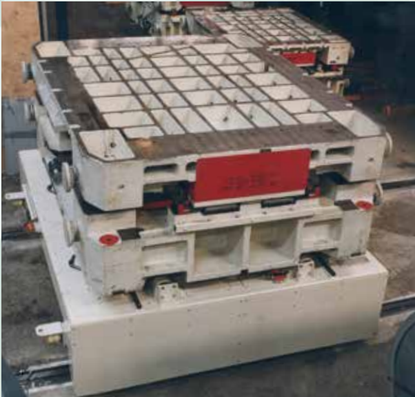
1 x 18 ton die change car on rails.
