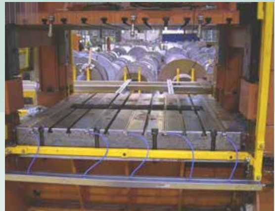
Pneumatic operated die lifters. Easy to install, easy to remove
