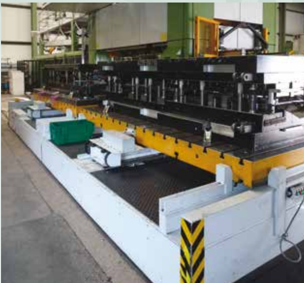
1 x 18 ton die change car on rails.
