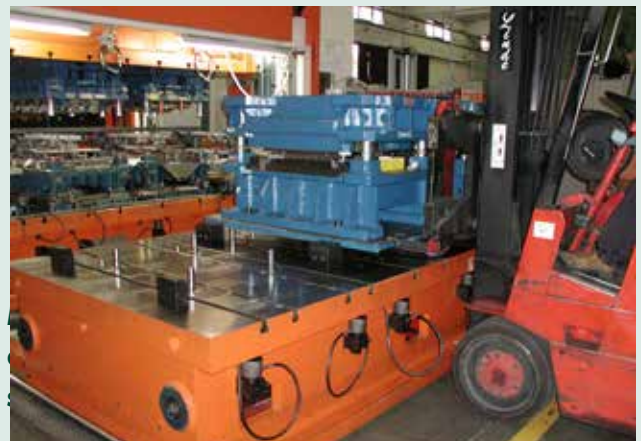
Bolster with air operated die lifters, pre rollers, ECA cylinders and parking stations.
